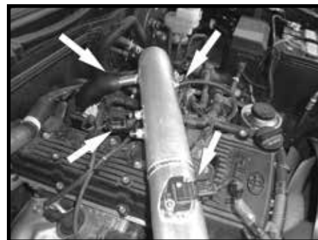
Step 15 Connect the fuel pressure regulator hose, and the crank case vent hose to the intake tube. Connect the mass air sensor electrical connection as shown. Install the pressure sensor onto the Spectre intake using the bolts removed in Step 3.
