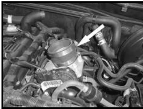
Step 11 Install the provided coupler onto the throttle body and secure with the provided hose clamps.
