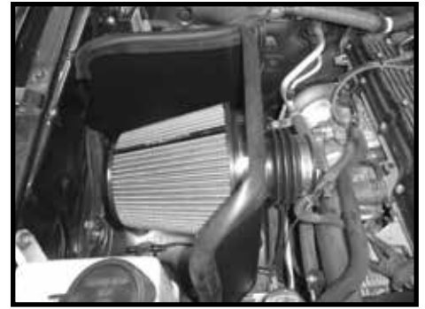
Step 10 Install the filter onto the heat shield using the 3" flex coupler and the provided hose clamps as shown.
