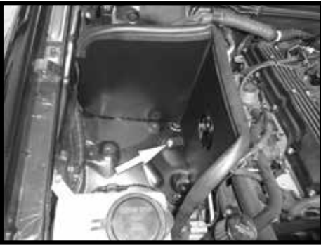
Step 8 Install the heat shield and secure it using the provided hardware.
