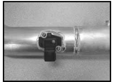
Step 13 Install the mass air sensor into the Spectre intake tube and secure with the provided hardware.
