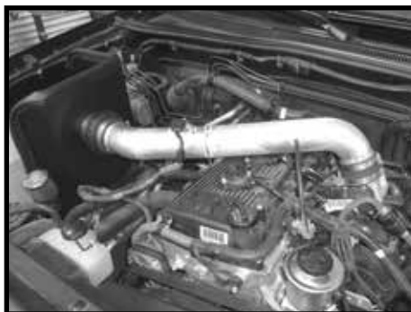
Step 14 Install the Spectre intake tube onto the throttle body and into the flex coupler in the heat shield. Secure the tube by tightening the hose clamps at the couplers.
