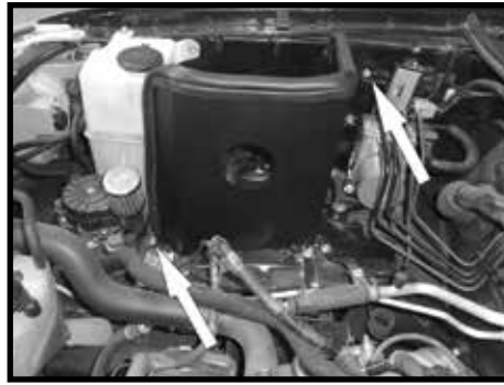
Step 9 Secure the heat shield using the stock hardware in the 2 places as shown.
