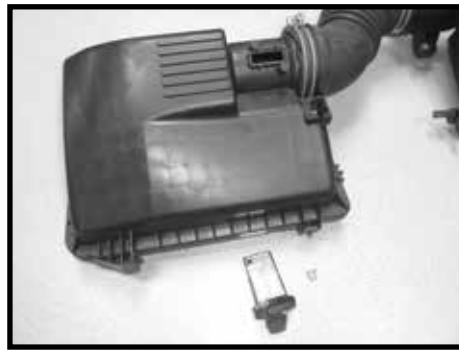
Step 12 Remove the 2 mass air sensor retaining screws and then remove the mass air sensor from the factory air box.
